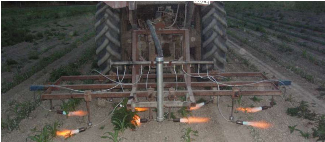
I Figure 30. Selective, intrarow flame weeder working in sweetcorn
