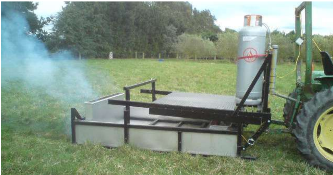
I Figure 29. A bed flame weeder for stale seedbeds
